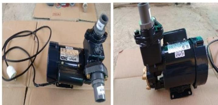
**Gambar 3.** Pompa Isap *Shimizu* 120 *Watt*
