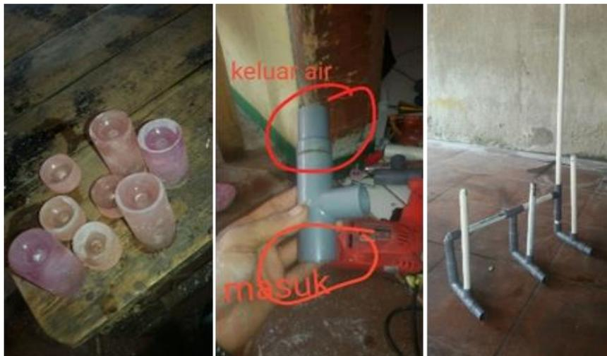
**Gambar 2.** *Nozzel Micro Bubble*
