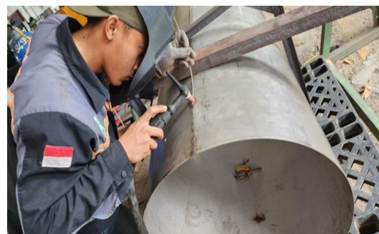
(b). Welding tabung reaktor
